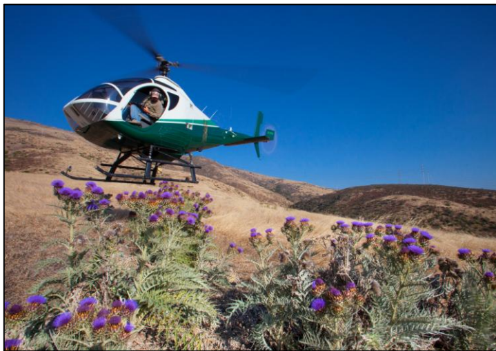
Figure 2. Botanical surveyors demonstrating ease of detection and maneuverability at 15-feet altitude in a Schweizer-333 turbine-helicopter.
